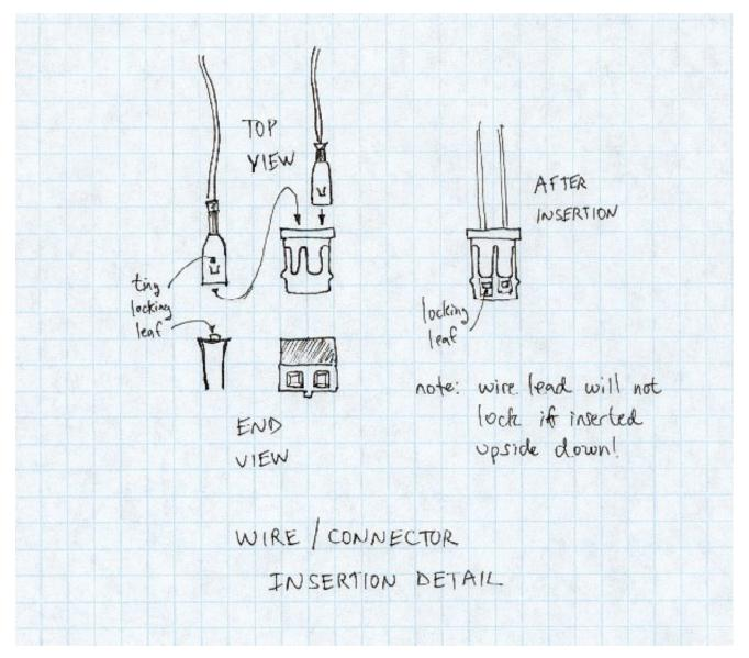
When the lead is inserted correctly, you will feel a tiny "click" as the connector locks itself into the plug. If it is inserted upside-down or side-ways, the connector won't lock and you can pull it out and try again.
